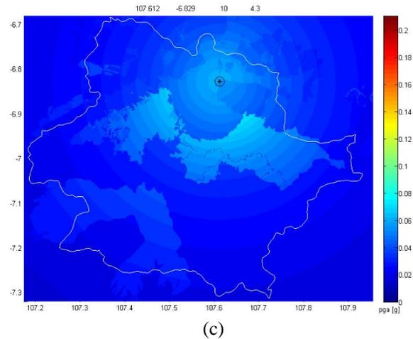
Fig5. PGA for single event for a) maximum scenario b) medium scenario c) minimum scenario Simulations show that the most affected area beside around Lembang fault area is the south of Bandung city. It is because lacustrine sediment in southern area.
